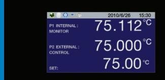
Displays calibration temperatures to 1/1000 degree C.
