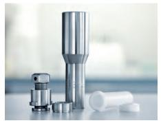
**Materials that are difficult to digest** or high sample weight represent a challenge for modern digestion instruments. Digestec by Berghof is distinguished by its high working pressure of up to 200 bar and offers the ideal solution for the most difficult samples. The decisive plus points are its simple filling and a digestion carried out under uniform heating that can be reproduced at any time.
